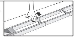
Once all screws are started, you can now tighten all of the Machine screws, and secure the center rails using the M6x10 Machine screws. Resume your desk instructions from here!
