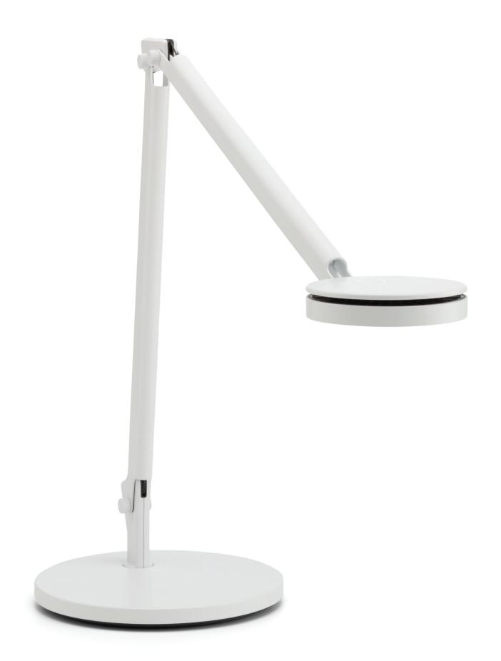
The dash task light has the distinction of being the first freestanding LED task lamp to achieve BIFMA Level 1 certification. It is 97% recyclable with 32% recycled content. Other sustainability features include mercury-free LEDs and a wireless electrical current that eliminates the use of PVC. The low-energy 8-watt LED array is easily replaceable after 50,000 hours or when new technology becomes available—whichever comes first.
