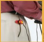
A magnetic safety clip attaches to the user and automatically shuts off the treadmill if the magnetic connection
