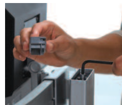
To change height setting use built-in Allen wrench or 5/32" drill bit.
