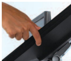
Unique counter-balance spring offers easy two-fingered "feather-touch" tilt adjustment. Monitor tilts 90° to allow instant access to connections.
