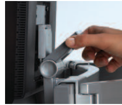
VESA connection cover conceals both the mount and security feature to maintain a clean profile.
