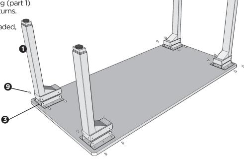
**D.** Attach the four (4) Small Feet (part 2) to the four (4) Legs (part 1), each with four (4) Machine Screws (part 9).
