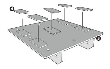
**B.** Place each Zero Crossbar Bracket (part 3) on the underside of the desktop. Carefully measure from all sides and attach the Zero Crossbar Brackets (part 3) to the underside of the desktop with twenty-four (24) Pan Head Screws (part 10), six (6) per bracket.
