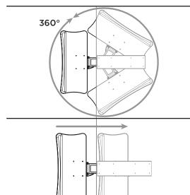
The Keyboard Tray rotates at the point where the Mechanism attaches to the Track. It can rotate 360 degrees.
