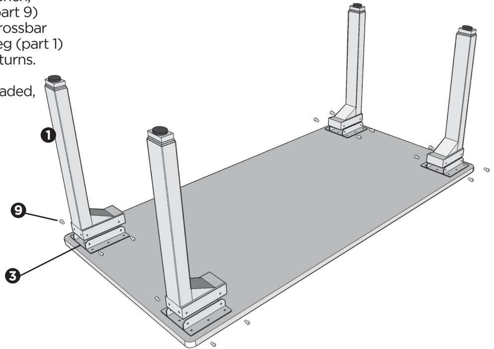
**D.** Attach the four (4) Small Feet (part 2) to the four (4) Legs (part 1), each with four (4) Machine Screws (part 9).
