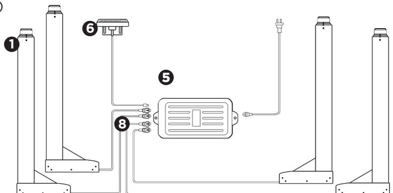
F. Attach the Control Box (part 5) to the underside of the desktop using two (2) M5x16 Screws (part 10). Ensure it is placed close to the center of the desktop so the cables can reach it.
