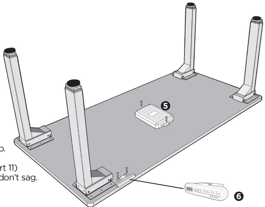
**i** If your desktop is not pre-drilled, we recommend that you pre-drill the holes for connecting the Control box (part 5) and Keypad (part 6) to the desktop. Drill 1/2" deep (max) with a 1/8" drill bit. Never use countersunk screws.
