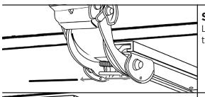
**Step 4** Lift up on the front of the tray and lower the back to relieve pressure on the shipping pin and remove it.
