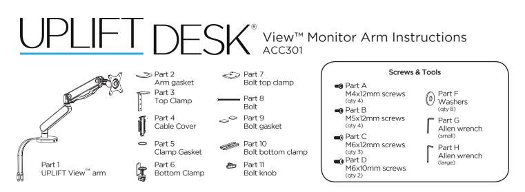
There are two ways to attach your UPLIFT View<sup>™</sup> Monitor Arm to your desktop: Clamp and Bolt-thru assembly.
