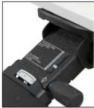
Built in height and tilt gauges allow evaluators to set and record position.
