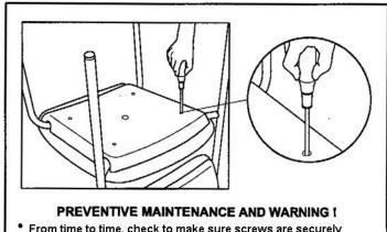
From time to time, check to make sure screws are securely tightened. Holes on PP shell are for convenient checking.
