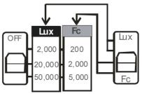
Example: If a measurement on the 5000 Fc range displays 350, then the actual measured value is:  $350 \times 10 = 3500 \text{ Fc}$ .
