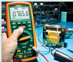
Measure the insulation resistance of transformer windings
