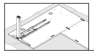
Line up the first Leg assembly with inserted rails to the outer pre-drilled holes on the Main desktop.
