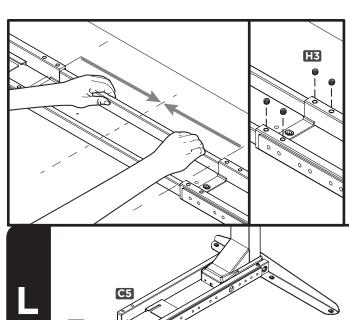
Slide the Crossbar rail (C6) and Open crossbar rail (C13) until the Center indicator mark is in the middle. Once this is done, the Crossbar rail will be centered, and in the proper position.
