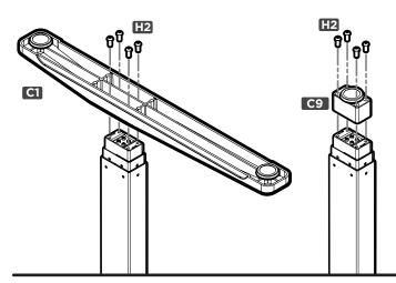
When you've decided, attach the feet to the legs. Make sure the long end of the Feet (C1) are pointing towards the inside of the L-Shaped desk, in the same direction as the Side brackets.
