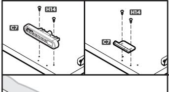
Attach the Keypad to the outermost end of the Return desktop. There are two sets of holes to accommodate different Keypads. Line up your Keypad (C7) with the pre-drilled holes, and attach it to the Desktop with two #10x5/8" Wood screws (H14).
