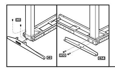
Place all leg assemblies upside down. For the first two, insert the Side brackets (C2) tabs inside the Crossbar end, and attach using two M6x10 screws (H1).
