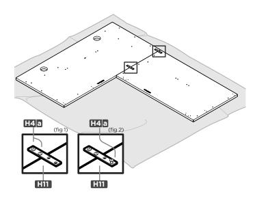
Make sure both Main and Return desktops are flush. Line up the Support brackets (H11) over their corresponding pre-drilled holes.
