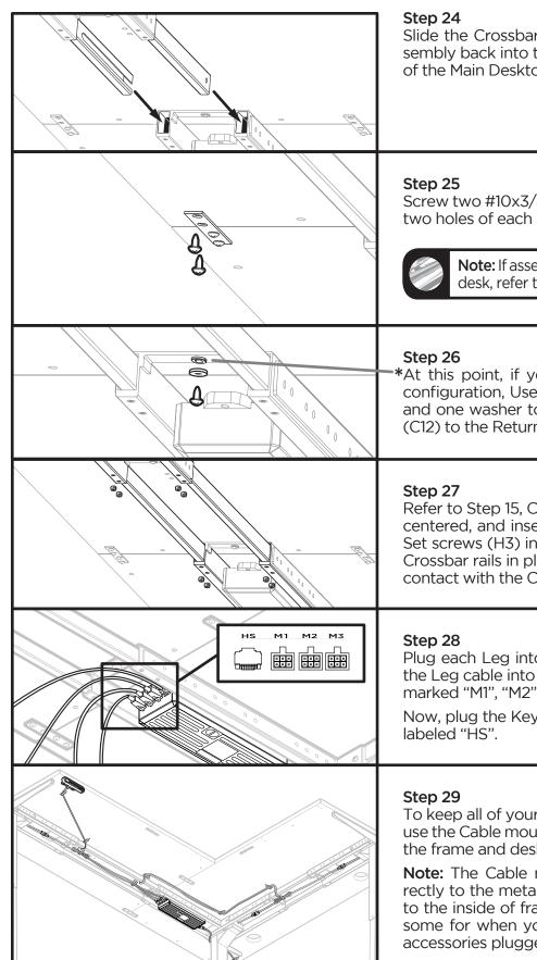
Slide the Crossbar rails from the Return desktop assembly back into the Long corner crossbar end (C12) of the Main Desktop assembly.
