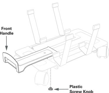
**Step 2:** Attach Front Handle by placing bolt through one of three holes on base (depending on desired handle extension) and secure with plastic screw knob.
