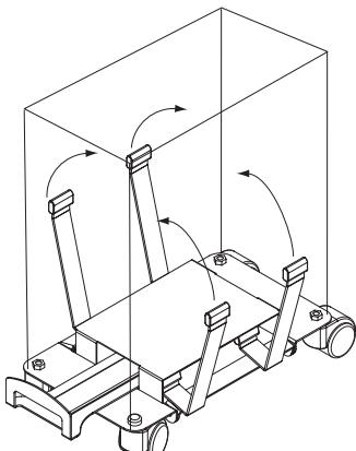
**Step 4:** Center CPU on platform. The arms will automatically close to secure the CPU in place.
