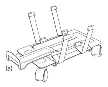
**Step 1:** Open arms of CPU Dolly and attach Front Handle (a) as shown by placing bolt through one of three holes on base (depending on desired handle extension) and attaching plastic screw knob to bolt.
