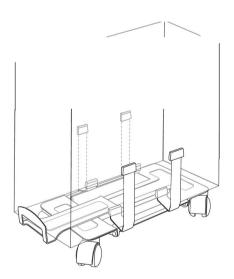
**Step 2:** Place CPU into unit. The arms will automatically close to secure the CPU in place.
