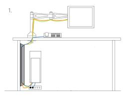
Install the small-diameter 24" channel vertically, by nearby wall outlet or CPU.
