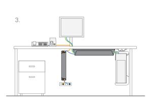
Install the large-diameter 24" channel horizontally, below desktop. Position small-diameter 17" channel vertically by nearby wall outlet or CPU.
