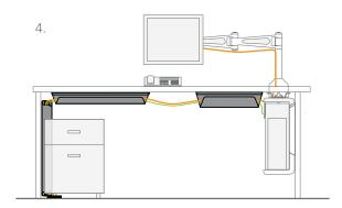
Install the large-diameter 17" channel and small-diameter 24" channel horizontally, from end-to-end, below desktop. Position second small-diameter 24" channel vertically, above floor outlet.
