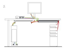
Install the large-diameter 17" channel and small-diameter 24" channel horizontally, from end-to-end, below desktop.
