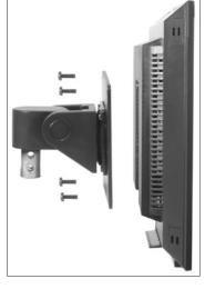
Align the tilter and VESA bracket with the hole pattern on the back of the flat panel monitor.
