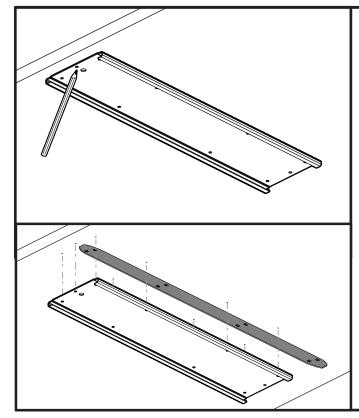
If you are not using the Track Spacer Kit, place the Track underneath your desktop in the desired location, with about 1/2" from the front edge of the desktop to the front edge of the Track.\* Using the Track as a template, mark the center of the holes with a pencil (ten holes on a 21" Track and eight holes on an 11" Track).
