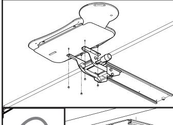
For the Switch Tray: Attach the Tray to the Mechanism by lining up the integrated screws on the bottom of the Tray with the holes on the Mechanism; secure in place by attaching the four Acorn nuts onto the screws from below.
