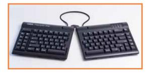
A flexible pivot tether connects both modules allowing an infinite range of splay and greatly reducing ulnar deviation.
