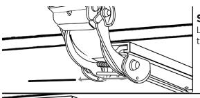
**Step 4** Lift up on the front of the tray and lower the back to relieve pressure on the shipping pin and remove it.
