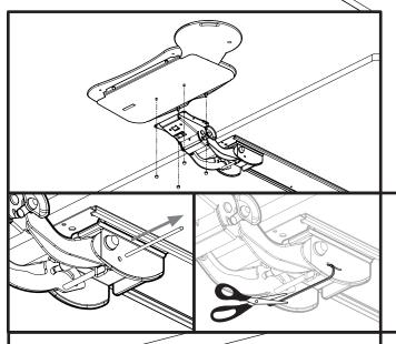
up the integrated screws on the bottom of the Tray with the holes on the Mechanism; secure in place by attaching the four Acorn nuts onto the screws from below.
