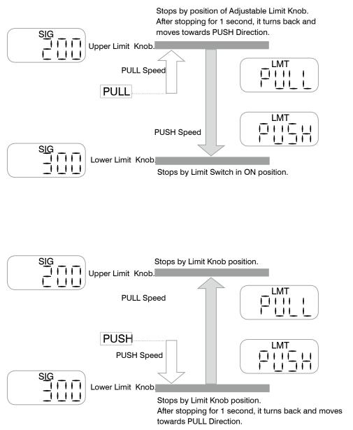
Change speed by UP, DOWN Key. SIG Mode and CON Mode Speed Setting are commonly used. During movement, Speed variation is not possible. When no movement is occurring (at idle), the display shows movement Mode and the latest operated speed. When the movement starts, the respective memorized movement speed is displayed.
