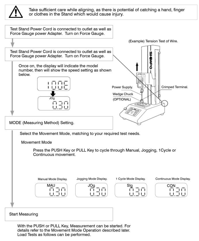
Press Test - Tensile Strength Test - Weld Strength Test - Peel off Test - Absorption Power Test Resistance Power Test - Uncapping (Seal) Test - Punching Test.
