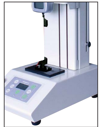
Stand with Optional Grip Performing Tension Test
