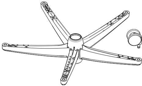
Place the 5 star base upside down and install the casters by firmly pushing the metal stem into the appropriate pocket until fully seated.
