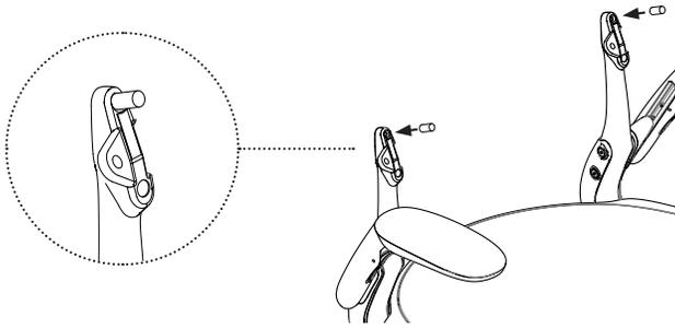
Install the hard foam parts on both sides of the seat frame.
