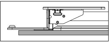
Keep the unit in a position so that the Keyboard Tray rests ON the desktop when in the lowest position, to prevent any risk of the unit tipping forward
