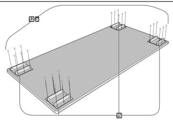
**C1.** Using the supplied Allen wrench, insert four (4) M6x14 Machine screws (part 10) through the holes in each Zero crossbar bracket going into the Leg (part 1) and rotate each screw just a few turns.
