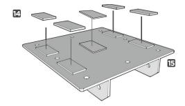
**B1.** Carefully measure from all sides, and place each Zero crossbar bracket (part 15) on the underside of the desktop. Attach the Zero crossbar brackets to the underside of the desktop with twenty-four (24) #10x5/8" wood screws (part 12-a), six (6) per bracket.
