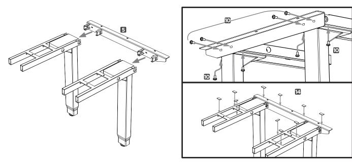
**D.** Insert the Crossbar rails (part 4) into the Crossbar ends. Ensure that they are facing inward, with the slot closer to the underside of the frame, or else they will not insert properly.
