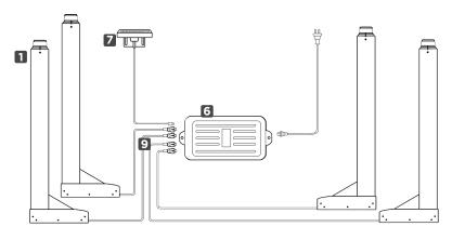
I. Place the Control box (part 6) in a spot where all wires (from the previous step) can reach. Use two (2) #10x5/8" wood screws (part 12-a) to affix it to the desktop.
