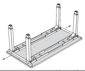
**F.** Lock the position of the Crossbar rails using sixteen (16) M6x10 machine screws (part 11) to keep everything in place. Ensure that the machine screw hits the metal of the Crossbar rail to keep the assembly from moving.
