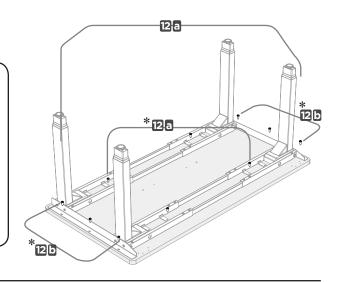
**H.** Using the cables (parts 9), connect the Legs (part 1) to the Control boxes (part 6) and the Keypad (part 7) as per the diagram here.
