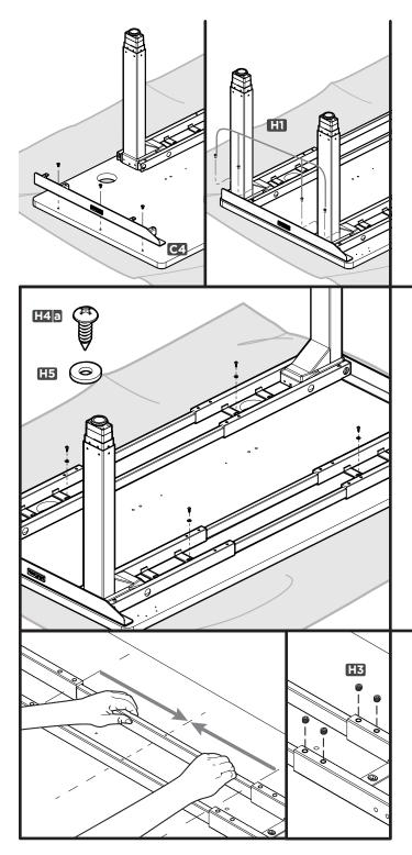
Align the holes in the second Side bracket (C4) with the pre-drilled holes or threaded inserts on the other side of the Desktop. Once again, make sure that the beveled edge of the Side bracket is pointed towards the front of the Desktop. Then attach it with three of the screws chosen in Step 4.
