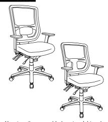
Now turn the assembled seat upright and locate the center hole of the Mechanism over the Seat Post. Push down firmly until the connection is secure.
