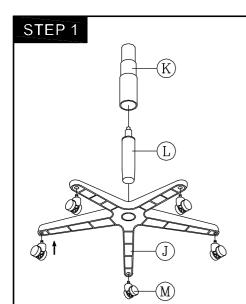
Press the Casters (M) into the holes at the end of each leg of the Base (J). Insert the bottom end of the Seat Post (L) into the center hole of the Base (J). Slide Seat Post Cover (K) over the Seat Post (L).
