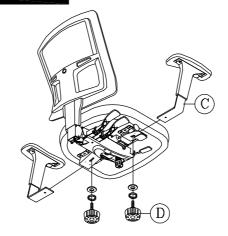
To attach your armrests, insert Left and Right Armrests (C) on the correct sides of the chair into the brackets located under each side of the Seat Cushion (B)
