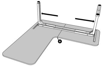
The desk feet are deeper than the side brackets. If your top is 25.5"-27.5" deep and you want the rear edge of the top in line with the rear edges of the feet, offset your desktop toward the back.
