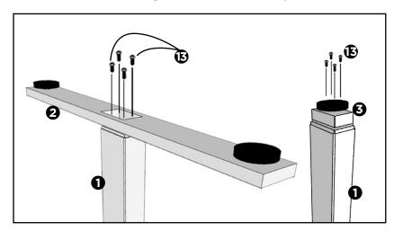
Your desktop may or may not be pre-drilled. Please check both sides of the desktop before placing the desk base on it for pre-drilling! Carefully place the upside down desk base on the underside of the desktop.
