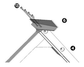
Remove backing from adhesive pads and position as shown: five adhesive pads each for the brackets, crossbar ends, and zero crossbar bracket.
