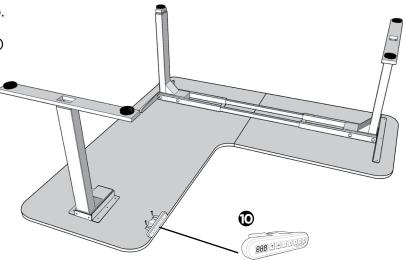
**N.** Turn the assembled desk right-side-up. With two people, grab the desk by the base (not the desk top) and turn the desk right-side up. Adjust the Leveling Studs on the Feet (Part #2) as needed.
