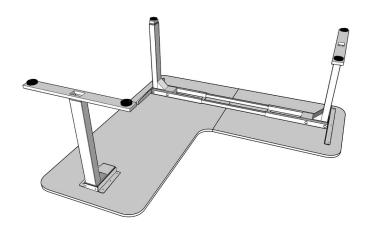
**J.** Double-check that the base is centered on the underside of the desktop and is located where you want it. Also, double-check that the included wood screws are not too long for your desktop and won't puncture the surface when screwed all the way in.
