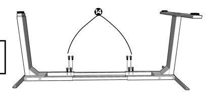
Place the 1-leg base assembly (this should be the remaining Crossbar End and Leg assembly with Long Side Bracket). Location will vary depending on the size and shape of your desktop. Choose the location that provides the most balance to the desk. Match the alignment you selected for the 2-leg base assembly.
