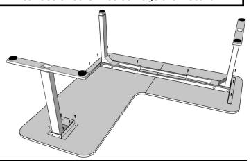
**K.** Using the wires, connect the Legs (part 1) to the Control box (part #9) and the Keypad (part #10) Wires as per the diagram below.
