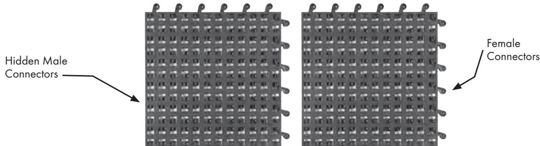
**Step 2 (a).** Lay the second tile over the first, placing the female side over the male interlocks. Using a rubber mallet, secure the tiles together. Repeat this process completing one row at a time.
