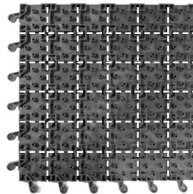
Tiles can be cut every 3" and still connect. For best results, flip the tile upside down. Cut along lines as indicated in the photo. The line equally bisects the circular support. To modify tiles to fit around an object or other impediment, it is not necessary to flip the tile over. Simply measure and cut along the surface.
