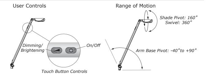
On/Off: Press and release the On/Off button once to turn on or off. Note: The lamp will
